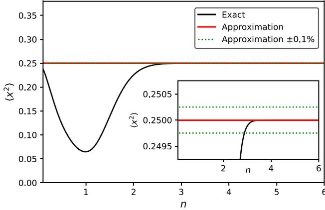
FIG. 5. The exact mean-squared displacement is calculated as a function of  $n$  for a quadratic background energy landscape.  $Q = 2$ ,  $m = 2$ ,  $\alpha = 4$ .
