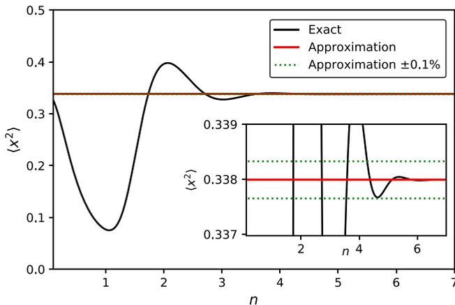
FIG. 6. The exact mean-squared displacement is calculated as a function of  $n$  for a quartic background energy landscape.  $Q = 2$ ,  $m = 4$ ,  $\alpha = 4$ .
