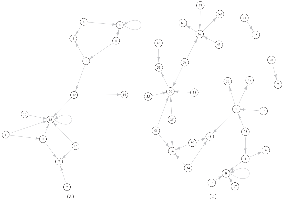
FIG. 7. State transitions graphs for (a) \mathcal{A}_4 and (b) \mathcal{A}_6 , trimming threshold is \theta = 0.2 . Nodes are labeled by digital representation of 4-bit (a) and 6-bit (b) states, respectively.
