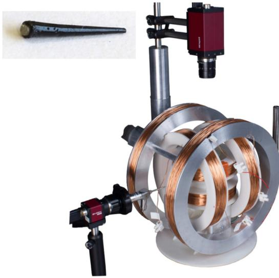
FIG. 1. Experimental setup [20]. The three orthogonal Helmholtz coils generate a homogeneous magnetic field in the center, where the swimmer has been placed. The swimmer is tracked using two perpendicular cameras. In the corner: Scaled-up flexible magnetic swimmer used in the experiments.
