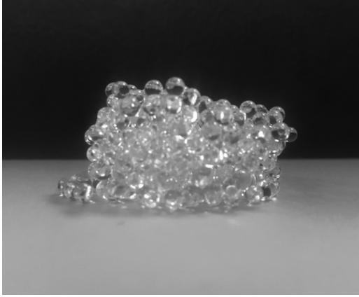
FIG. 1. Example of a cohesion-controlled granular material: a pile of glass beads d = 3 mm with a PBS coating layer of thickness b = 2.2 \mu\text{m}
