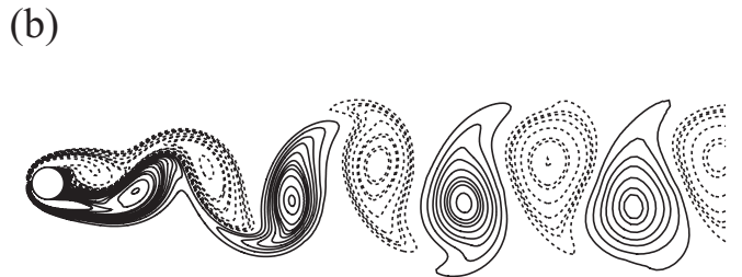
FIG. 4. (a) Time histories of lift and drag coefficients and (b) vertical contours (solid lines for positive values and dashed lines for negative values) for the flow around a circular cylinder at Re = 100 .
