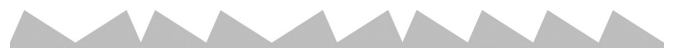
FIG. 2. A realization of the ratchet potential used in the numerics. The two possible orientations of each ratchet are chosen with equal probability.
