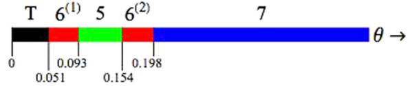
FIG. 9. Phase plot for l = 7 for the case that the system parameter a is positive while b and c are negative. For increasing \theta and t_7 negative, the system passes from a tetrahedral state to a state with a single sixfold symmetry axis, a fivefold axis, again a sixfold axis, and finally a sevenfold axis. The loci of the transition points are independent of t_7 .
