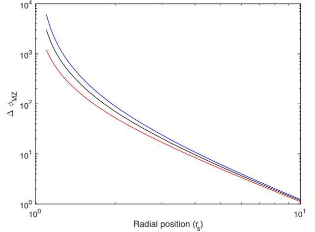
FIG. 5. Measured phase differences of  $L = 1$  m and  $h = 1$  m Mach-Zehnder interferometer near a black hole of Schwarzschild radius  $r_s = 10$  km, angular momentum  $a = \frac{r_s}{8}$ , and the operating frequency of light  $k = 2 \times 10^6$  m $^{-1}$ . Here we have the MZ phases for comoving (red), countermoving (blue), and no rotation  $a = 0$  (black).
