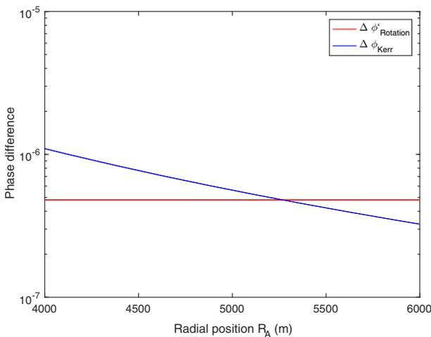
FIG. 4. Measured phase differences of  $L = 1$  m and  $h = 1$  m Mach-Zehnder interferometer around the radial position at which the Kerr phase (blue) becomes dominant on Earth compared to the phase due to the classical rotation (red).
