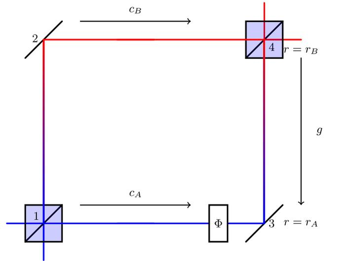
FIG. 1. A Mach-Zehnder interferometer of length  $L$  and height  $h$  stationary above the rotating planet.  $\Phi$  is a phase shifter in the bottom arm to calibrate the interferometer to a dark port of zero intensity.
