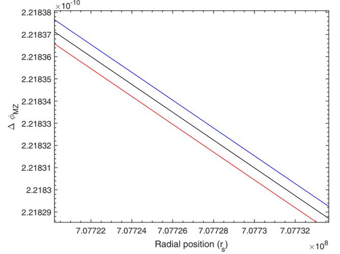
FIG. 2. Measured phase differences of  $L = 1$  m and  $h = 1$  m Mach-Zehnder interferometer in co- and counter-moving directions (blue and red, respectively). The black line is in the Schwarzschild metric with  $a = 0$ . We use the values for the Earth's Schwarzschild radius  $r_s = 9$  mm, rotation parameter  $a = 3.9$  m, and the operating frequency of light  $\omega = k = 2 \times 10^6$  m<sup>-1</sup>, corresponding to 500 nm measured locally at the source.
