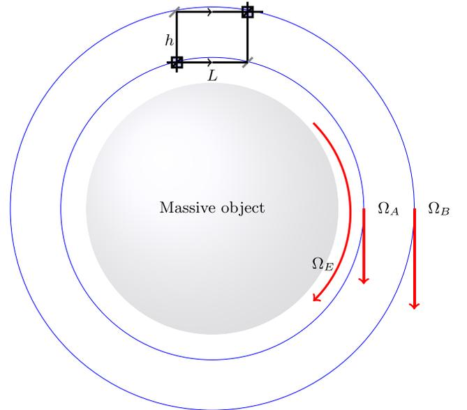
FIG. 3. A Mach-Zehnder interferometer of length  $L$  and height  $h$  stationary above the rotating massive object in the Kerr metric. Zero angular momentum ring-riders (blue) will have a locally flat space-time with  $c = 1$ . Their angular frequency as seen from a far-away observer (red) are given by  $\Omega_A = \frac{r_s a}{r_A^3}$  and  $\Omega_B = \frac{r_s a}{r_B^3}$ .
