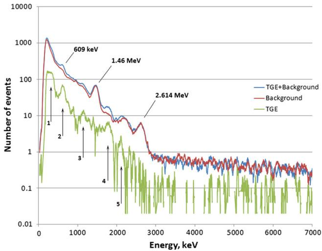
FIG. 2. Energy spectrum of the slowly varying, long part of TGE 17.08.2017 collected during the time interval 19:40–20:30. The background spectrum was derived for the time interval 17:40–18:30 of the same day. The numbers indicate lines from the Rn-222 daughter isotopes: (1) 242, 295, and 352 keV (unresolved); (2) 609 keV; (3) 1120 keV; (4) 1764 keV; (5) 2204 keV.
