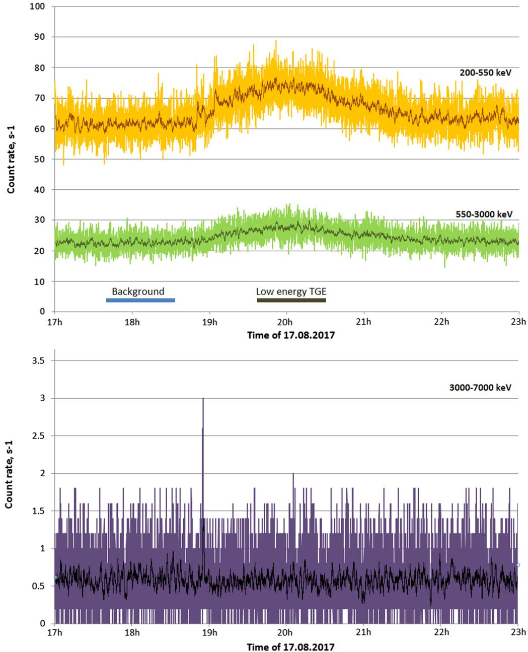
FIG. 1. Time profiles of TGE 17.08.2017 at different energy intervals, as measured at the Mount Aragats station by the gamma-ray spectrometer provided by SINP MSU.
