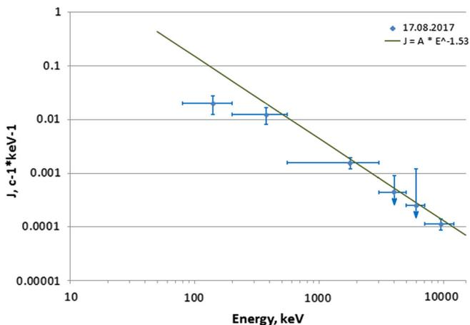
FIG. 4. Energy spectrum of the narrow peak of TGE 17.08.2017 taken for the period of time marked by the red line in Fig. 3.
