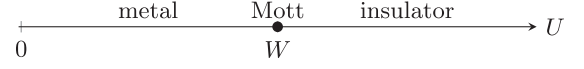
FIG. 1. Phase diagram of the HK model at zero temperature and half filling, as the interaction strength U is tuned from the noninteracting point U = 0 across the metal-insulator transition at U = W .
