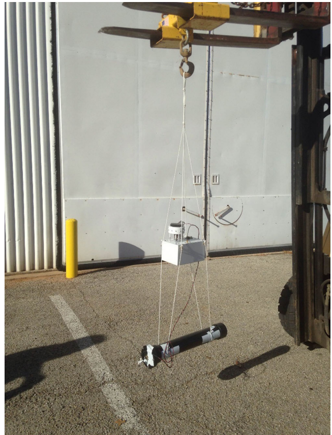
FIG. 5. Photo of HiCal payload taken during pre-flight hang test (June, 2016, Palestine, TX). Motor to drive piezo signal generator and transmitter antenna are enclosed within cylindrical pressure vessel, suspended from CSBF MIP electronics box. Pressure vessel was later painted white prior to flight.
