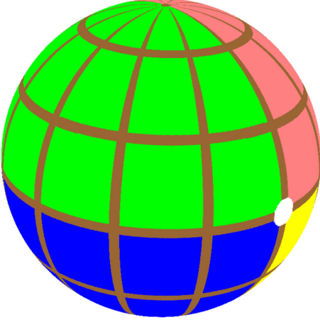
FIG. 1. The sphere light source marked by four different-colored quadrants and the brown grids of longitude and latitude. The white reference spot lies at the intersection of the four colored quadrants.
