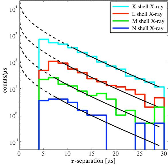
FIG. 6. Histograms of vertical separation (1  $\mu\text{s}$  is equivalent to 1.51 mm) between two vertices of EC events with the 203 keV gamma-ray emission for K-(cyan), L-(red), M-(green), and N-(blue) shell x rays. The distributions are fitted with the model described by Eq. (1). The solid black curves are the fits to data. The dashed black curves are the extrapolations from those fits.
