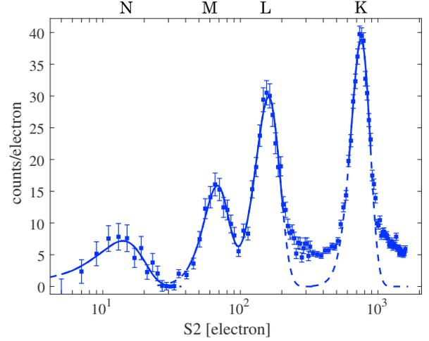
FIG. 7. X-rays' ER charge spectra. The S2 size has been converted to the number of electrons escaping recombination at the interaction site. The peaks from right to left are due to K-, L-, M-, and N-shell x rays respectively. The fits shown use Gaussian functions.
