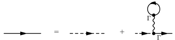
FIG. 2. The Dyson-Schwinger equation for the constituent quark mass. The dashed and solid lines stand for the bare and dressed propagators, respectively, and the vertex \Gamma = 1 . The wavy line represents the interaction.
