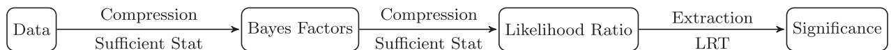
FIG. 1. Schematic of how information is compressed into a significance estimate within the oLIB algorithm. Ideally, sufficient statistics allow for lossless data compression, and the LRT allows for optimal information extraction.
