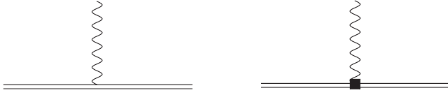
FIG. 1. The \mathcal{O}(p^2) and \mathcal{O}(p^4) tree-level diagram. The left dot and the right black square represent second- and fourth-order couplings, respectively.
