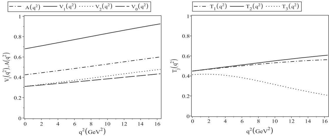
FIG. 3. The form factors  $A$ ,  $V_i$ , and  $T_j$  on  $q^2$ .
