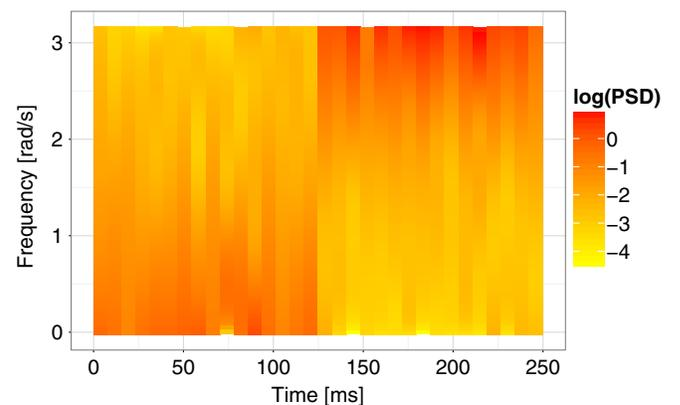
FIG. 10 (color online). Time-frequency map showing the estimated posterior median log PSDs for 32 segments of  $1/4$  s of AR(1) noise. The change-point in spectral structure occurs exactly halfway through the series.
