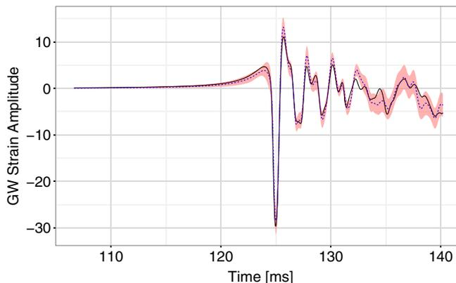
FIG. 3 (color online). Reconstructed rotating core collapse GW signal. The 90% credible region (shaded pink) and posterior median signal (dashed blue) are superimposed with true *A1O12.25* GW signal from the Abdikamalov *et al.* [25] test catalogue (solid black).
