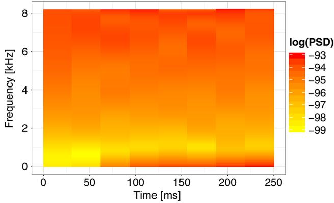
FIG. 14 (color online). Time-frequency map of the estimated time-varying noise spectrum for 8 segments of 1/4 s simulated Advanced LIGO noise. The posterior median log PSDs for each noise segment are used.
