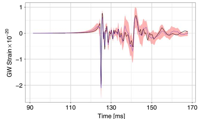
FIG. 13 (color online). Reconstructed rotating core collapse GW signal. The 90% credible interval (shaded pink) and posterior mean (dashed blue) are shown, overlaid with the true A1O10.25 signal (solid black) from Abdikamalov *et al.* [25] test catalogue. The signal is scaled to a SNR of  $\rho = 50$ .
