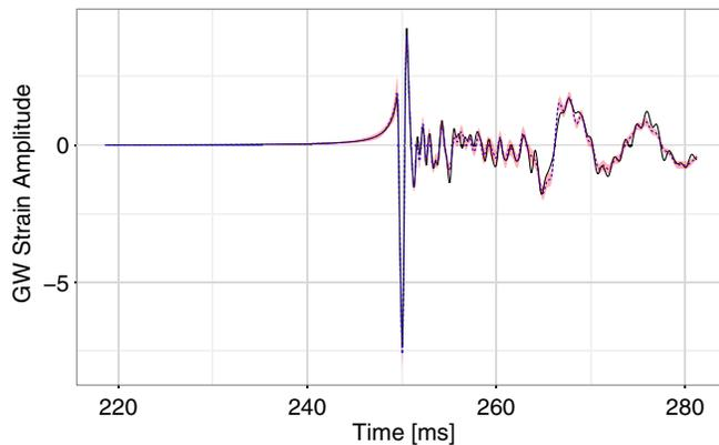
FIG. 9 (color online). Reconstructed rotating core collapse GW. The 90% credible region (shaded pink) and posterior median signal (dashed blue) are shown, superimposed with the true A1O8.25 GW signal from the Abdikamalov *et al.* [25] test catalogue. The first half of the signal was embedded in AR(1) noise with  $\rho = 0.5$ , and the second half had AR(1) noise with  $\rho = -0.75$ . Both noise segments had Gaussian white noise with  $\sigma_e^2 = 1$ .
