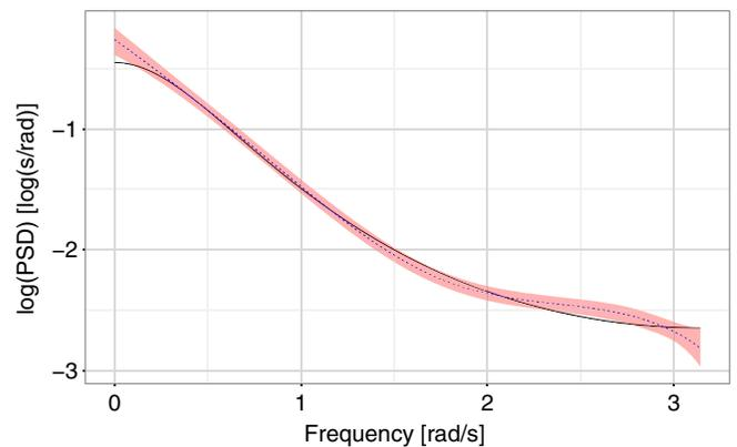
FIG. 7 (color online). Spectral density estimate of the first noise segment ( $\rho = 0.5$ ) from Fig. 6. The 90% credible region (shaded pink), posterior median log PSD (dashed blue), and theoretical log PSD (solid black) are shown.
