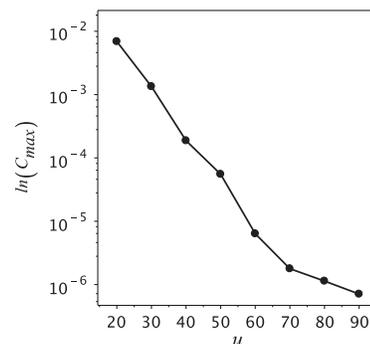
FIG. 1. Exponential decay of the maximum error in the global energy conservation with the increase of the truncation orders  $N$ .
