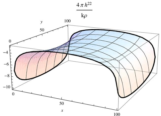
FIG. 5 (color online). The function  $\frac{4\pi}{k\rho}h^{22} = -[\phi_{(2)} + \phi_{(4)}]$  for a ring laser of side length  $a = 100$  units. The bold contour outlining the plotted area is at a distance of 1 unit from each side of the ring laser.
