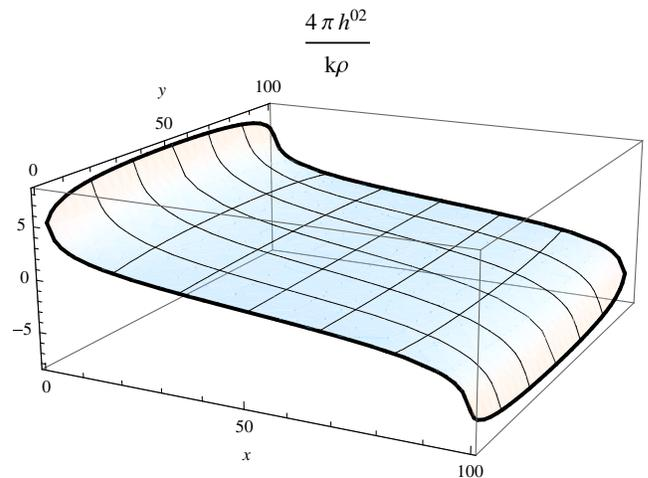
FIG. 7 (color online). The function  $\frac{4\pi}{\kappa\rho} h^{02} = -[\phi_{(2)} - \phi_{(4)}]$  for a ring laser of side length  $a = 100$  units. The bold contour outlining the plotted area is at a distance of 1 unit from each side of the ring laser.
