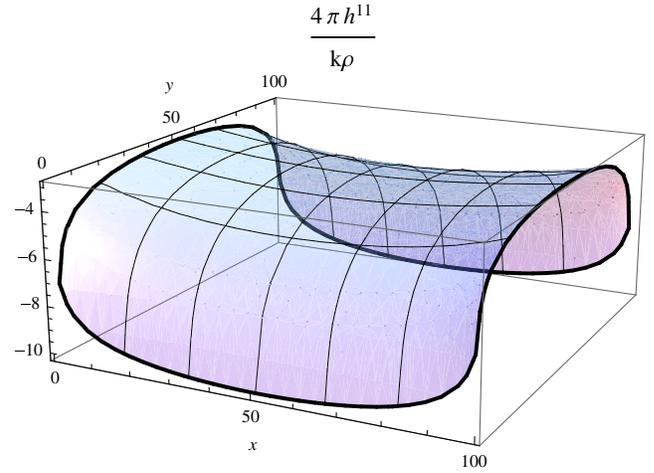
FIG. 4 (color online). The function  $\frac{4\pi}{k\rho}h^{11} = -[\phi_{(1)} + \phi_{(3)}]$  for a ring laser of side length  $a = 100$  units. The bold contour outlining the plotted area is at a distance of 1 unit from each side of the ring laser.
