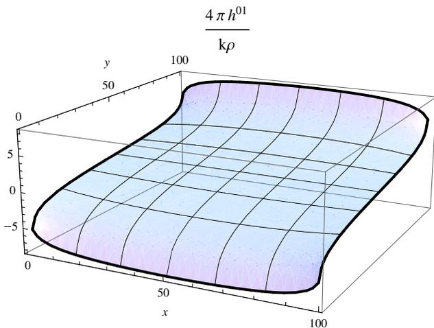
FIG. 6 (color online). The function  $\frac{4\pi}{\kappa\rho} h^{01} = -[\phi_{(1)} - \phi_{(3)}]$  for a ring laser of side length  $a = 100$  units. The bold contour outlining the plotted area is at a distance of 1 unit from each side of the ring laser.
