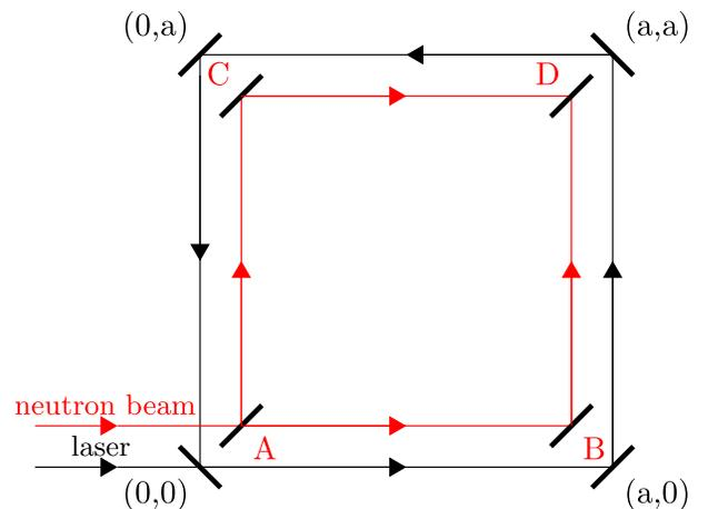
FIG. 2 (color online). Ring laser with side length  $a$  and interferometer.
