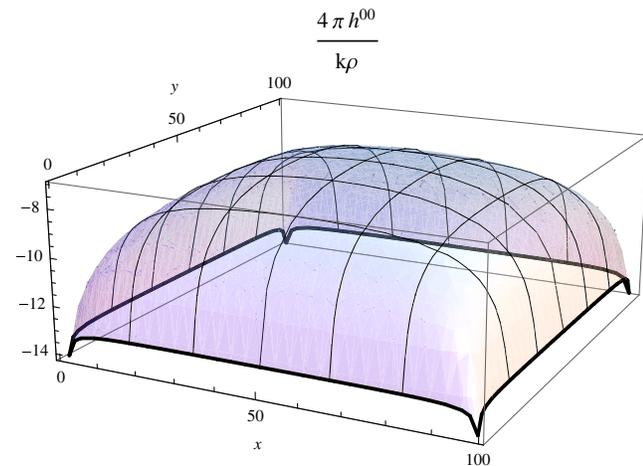
FIG. 3 (color online). Function  $\frac{4\pi}{k\rho}h^{00} = -[\phi_{(1)} + \phi_{(2)} + \phi_{(3)} + \phi_{(4)}]$  for a ring laser of side length  $a = 100$  units. The bold contour outlining the plotted area is at a distance of 1 unit from each side of the ring laser.
