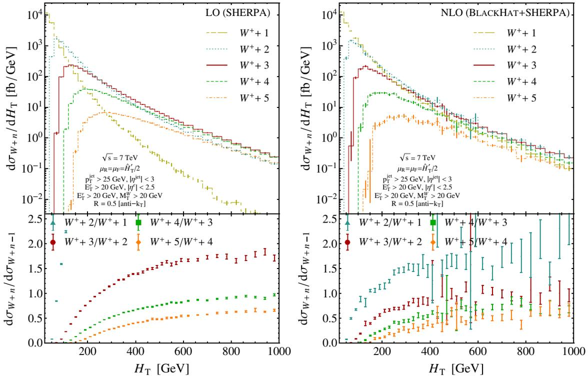
FIG. 12 (color online). The LO and NLO  $H_T$  distributions for  $W^+ + n$ -jet production at the LHC. The upper panels show the distributions in fb/GeV. From top to bottom, we display  $W^+ + 1$ -jet production through  $W^+ + 5$ -jet production. The lower panels show the jet-production ratios. The left plot shows the distributions and ratios at LO, the right plot those at NLO.
