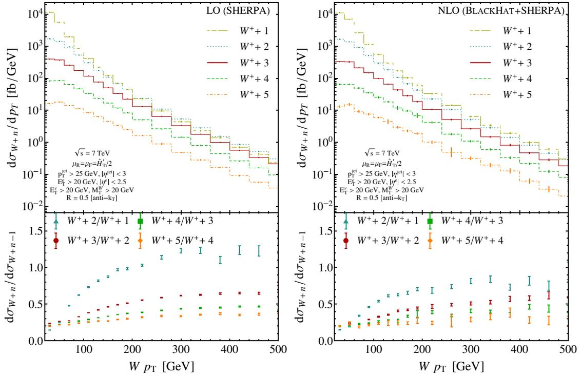
FIG. 8 (color online). The LO and NLO vector-boson  $p_T$  distributions for  $W^+ + n$ -jet production at the LHC. The upper panels show the distributions in fb/GeV:  $W^+ + 1$ -jet production through  $W^+ + 5$ -jet production are ordered from top to bottom. The lower panels show the jet-production ratios. The left plot shows the distributions and ratios at LO, the right plot those at NLO.
