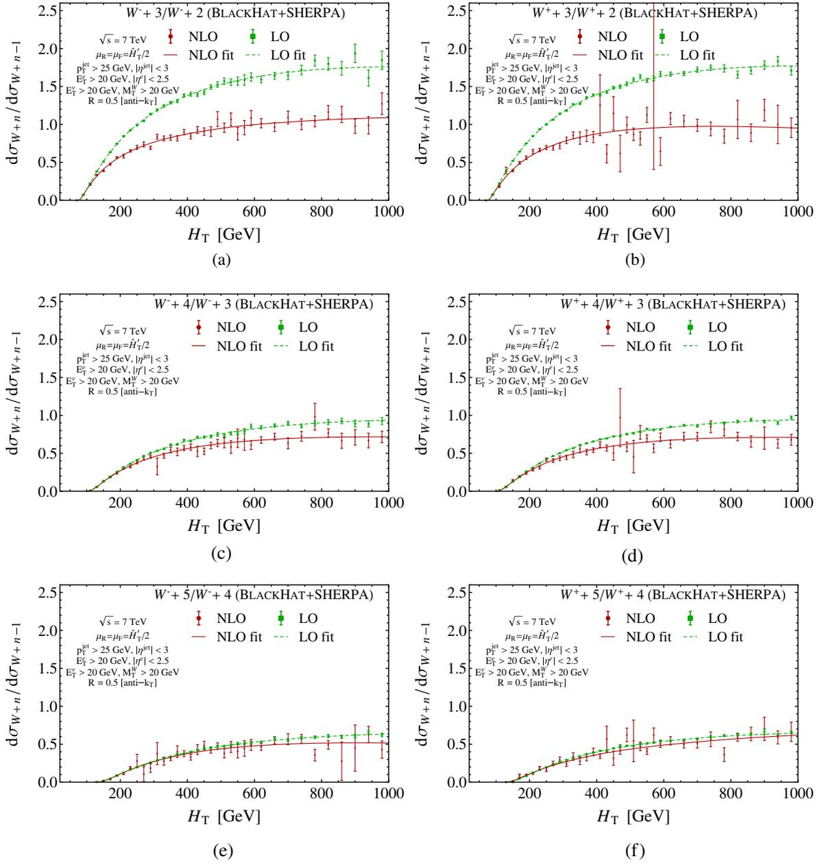
FIG. 13 (color online). Fits to the ratios of the  $W + n$ -jet to  $W + (n - 1)$ -jet differential cross sections as a function of  $H_T$ . Each plot shows the computed LO and NLO ratios, as well as fits with the parameters in Tables VI–VII. In the left column we show the ratios for  $W^-$  and in the right column those for  $W^+$ . From top to bottom,  $n$  goes from 3 to 5.
