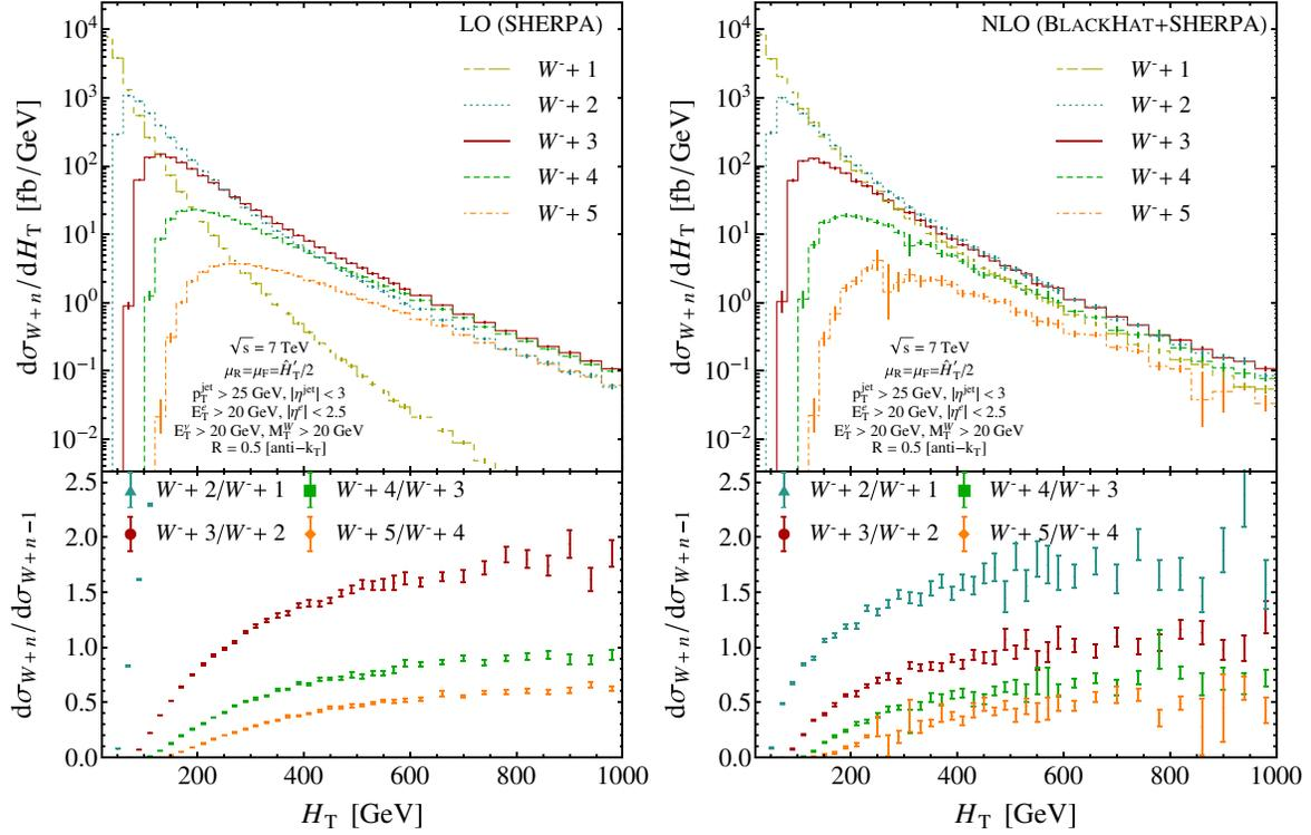
FIG. 11 (color online). The LO and NLO  $H_T$  distributions for  $W^- + n$ -jet production at the LHC. The upper panels show the distributions in fb/GeV. From top to bottom, we display results for  $W^- + 1$ -jet production through  $W^- + 5$ -jet production. The lower panels show the jet-production ratios. The left plot shows the distributions and ratios at LO, the right plot those at NLO.
