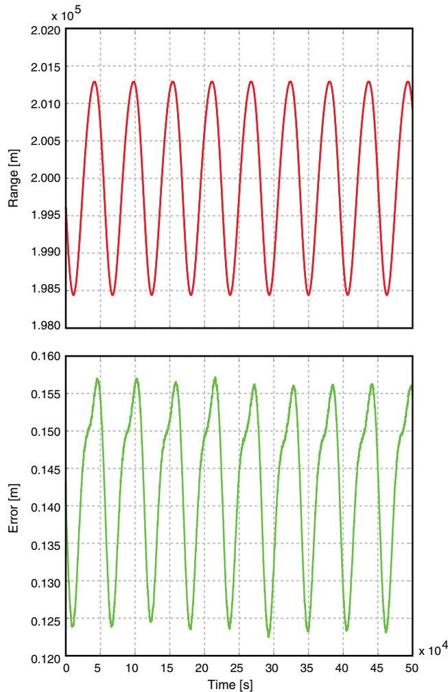
FIG. 6 (color online). The best guess of the interspacecraft range used to form the TDI combinations in Fig. 5. The simulated data used to find the best guess was from a  $5 \times 10^5$  s simulation sampled at 200 mHz. The range error, found by subtracting the known range from the fitted range, is plotted in the lower panel. The range error is an order of magnitude below the  $\pm 2$  m of the known range and therefore meets the timing requirements of the proposed GRACE-FO TDI experiment.
