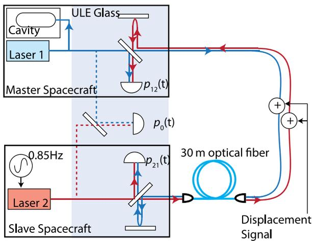
FIG. 8 (color online). Schematic layout of the TDIR experiment. The details of the injected displacement signal can be found in Fig 9.
