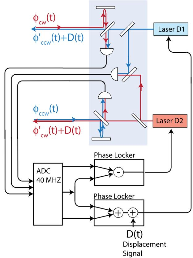
FIG. 9 (color online). Schematic layout showing the injection of the interspacecraft displacement signal. Three optical phase measurements are combined via two phase-locking algorithms to implement the required feedback combinations.
