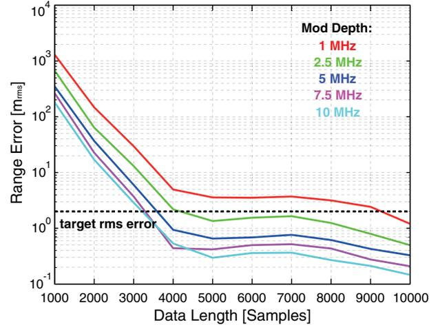
FIG. 7 (color online). The effect of varying data length and modulation depth in the tone-assisted TDIR algorithm. The rms range error can be seen to decrease as the data length increases or as the modulation depth is increased. For reference the 2 m rms ranging requirement needed to meet the timing requirements for a GRACE-FO TDI demonstration is shown. It can be seen that it is possible to meet this requirement for a range of data lengths and modulation depths.
