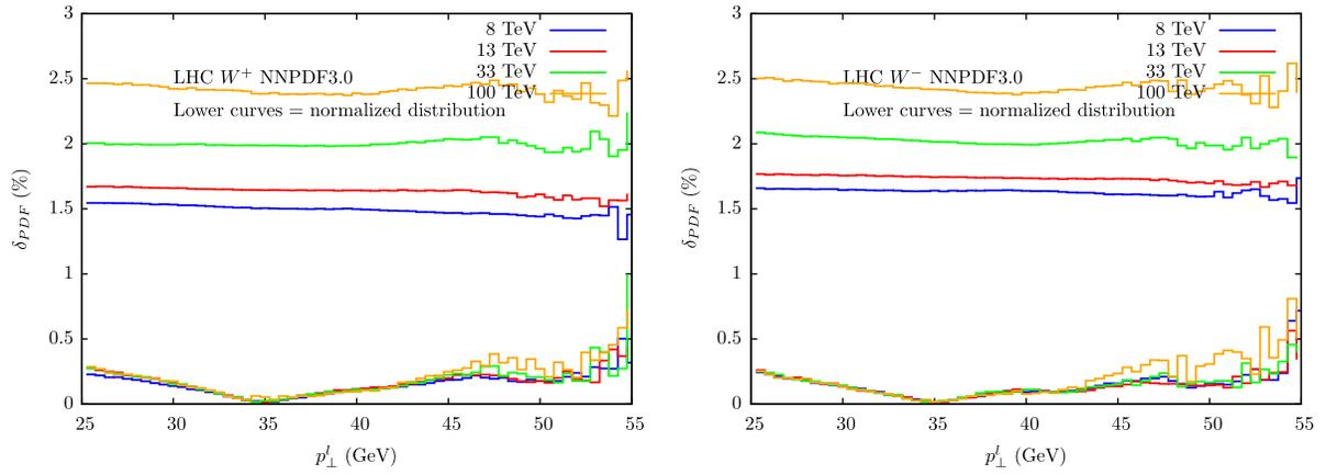
FIG. 3 (color online). Percentage size of the PDF uncertainty on the lepton transverse momentum distribution, computed with the NNPDF3.0 set at the LHC at different energies. Results for  $W^+$  (left) and  $W^-$  (right) production, in the case of absolute (upper lines) or normalized (lower lines) distributions.
