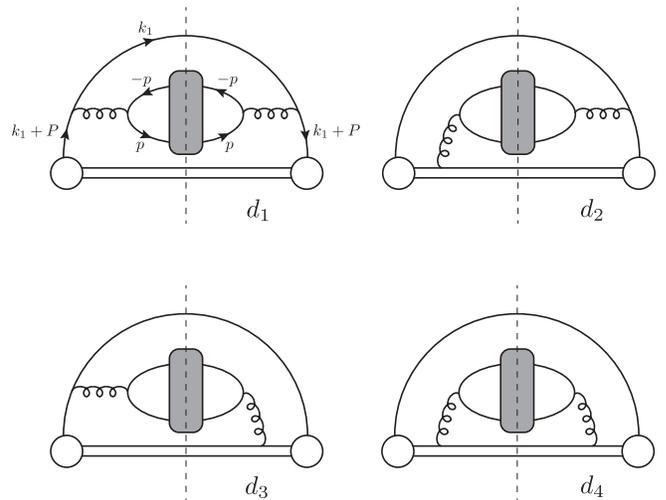
FIG. 1. Feynman diagrams for quark fragmentation into a color-octet  $Q\bar{Q}$  pair for the case in which the initial quark  $q$  and the quark  $Q$  that is a constituent of the quarkonium have different flavors. The diagram labels  $d_i$  correspond to the quantities that appear in Eq. (17).
