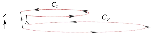
FIG. 2 (color online). A “shifted” double winding loop, in which contours C_1 and C_2 lie in planes parallel to the x - y plane, but are displaced from one another in the transverse direction by distance \delta z , and are connected by lines running parallel to the z -axis.
