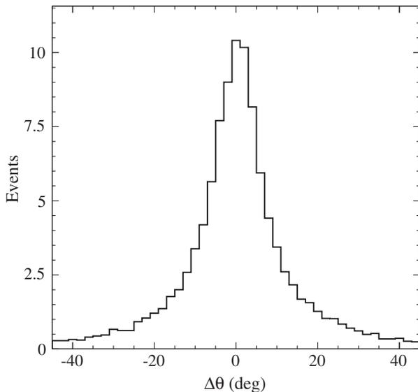
FIG. 6. The distribution of the difference between the true and measured antineutron polar angles at  $E_b = 960$  MeV.
