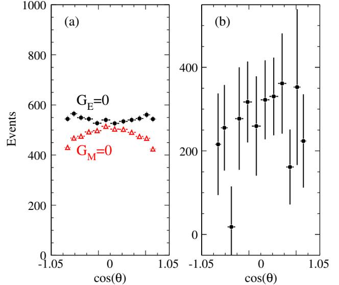
FIG. 7 (color online). (a) The  $\cos\theta$  distribution for simulated  $e^+e^- \rightarrow n\bar{n}$  events generated with  $G_E = 0$  and  $G_M = 0$ . (b) The  $\cos\theta$  distribution for data  $e^+e^- \rightarrow n\bar{n}$  events.
