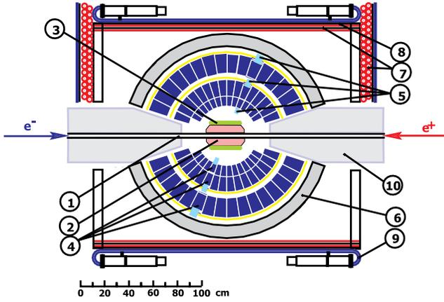
FIG. 1 (color online). Schematic view of the SND detector. The collider vacuum pipe (1) is surrounded by the tracking detector (2) based on a nine-layer drift chamber. The aerogel Cherenkov counter (3) provides  $K$  meson identification. The spherical electromagnetic calorimeter consists of 1680 NaI(Tl) crystals (4) with phototriode (5) readout. The muon detector (7)–(9) located after the iron absorber (6) provides muon identification and suppression of cosmic-ray background.
