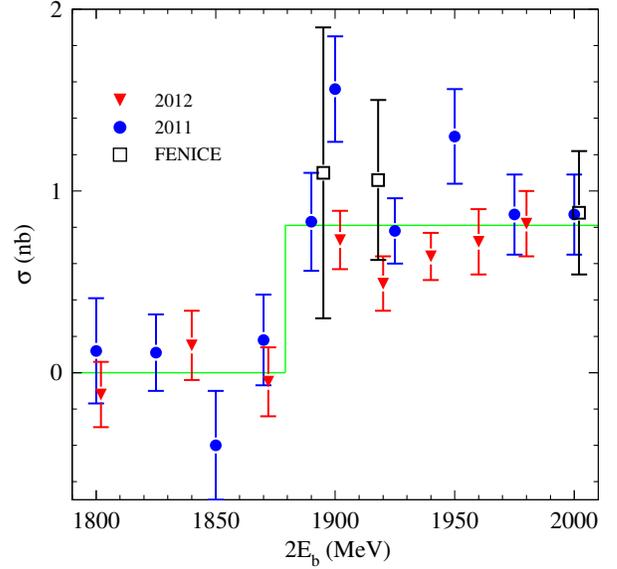
FIG. 9 (color online). The  $e^+e^- \rightarrow n\bar{n}$  cross section measured in this paper. The filled triangles represent 2011 data, while the filled circles correspond to 2012 data. The FENICE results [4] are shown by the empty squares. The lines below and above the  $n\bar{n}$  threshold indicate the average levels of the cross section. The quoted errors are statistical.
