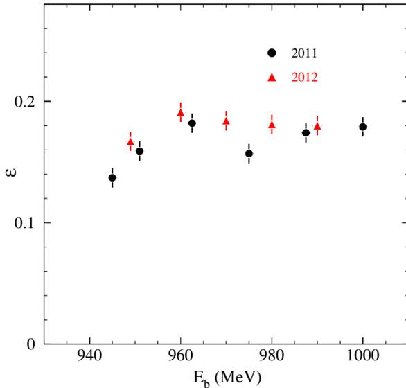
FIG. 3 (color online). The energy dependence of the detection efficiency for  $e^+e^- \rightarrow n\bar{n}$  events determined using MC simulation. The filled circles show the efficiency for the 2011 data set, and the triangles for 2012.
