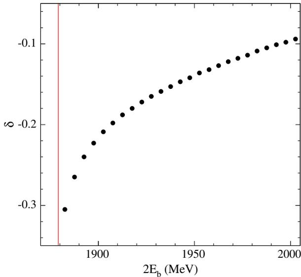
FIG. 8 (color online). The energy dependence of the radiative correction for the  $e^+e^- \rightarrow n\bar{n}$  process. The vertical line indicates the  $n\bar{n}$  threshold.
