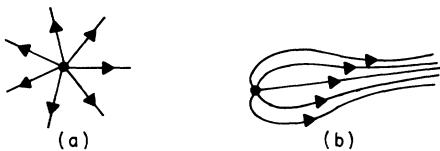
FIG. 2. (a) Flux lines associated with the spherically symmetric Coulomb field. (b) Distortion of the Coulomb field into a flux tube.
