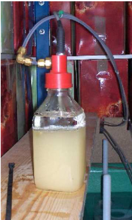
FIG. 2 (color online). Science C_2ClF_5 SDD during installation; the bottle is a squared 10 \times 10 \text{ cm}^2 base, 12 cm tall Schott glass containing \sim 900 \text{ ml} of freon + gel covered by a 6 cm glycerin layer. The cap contains the microphone and feedthroughs for the pressure (horizontal) and microphone (vertical) electronics.
