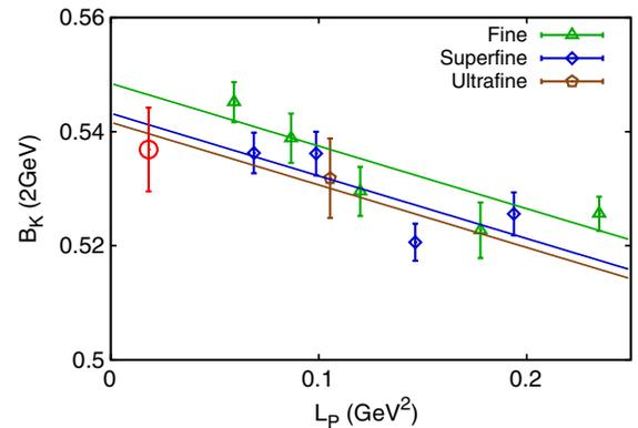
FIG. 2 (color online). Chiral-continuum extrapolation of  $B_K(\text{NDR}, 2 \text{ GeV})$ . The red circle shows the extrapolated result.
