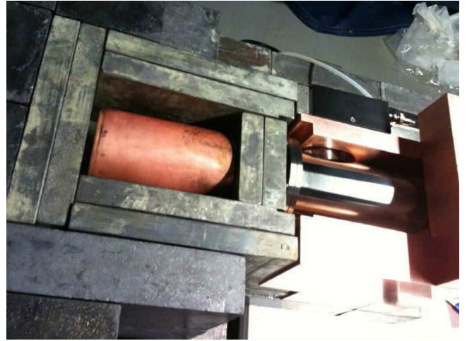
FIG. 1 (color online). Partially disassembled shield of the CoGeNT detector at SUL, showing the cylindrical OFHC end cap and innermost 5 cm of ancient 0.02 Bq ^{210}\text{Pb}/\text{kg} lead, characteristically oxidized following etching. The preamplifier is visible at the top right (black box). A minimum of 7 cm of lead thickness shields the detector from the naturally occurring radioactivity in the preamplifier's electronic components.
