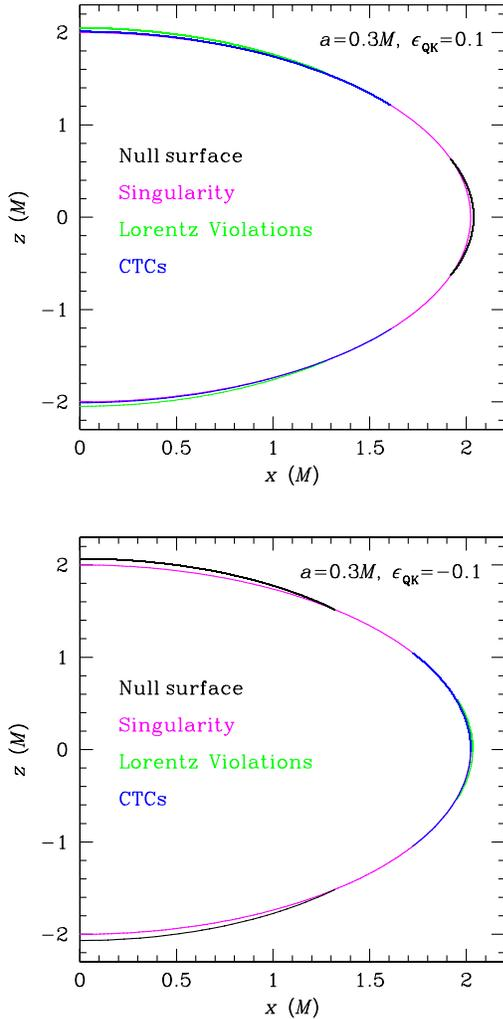
FIG. 6 (color online). Null surface and regions with Lorentz violations and closed timelike curves in the QK metric for  $a = 0.3M$ . Top panel:  $\epsilon_{\text{QK}} = 0.1$ ; Lorentz violations and closed timelike curves occur around the poles. Bottom panel:  $\epsilon_{\text{QK}} = -0.1$ ; Lorentz violations and closed timelike curves occur near the equatorial plane.
