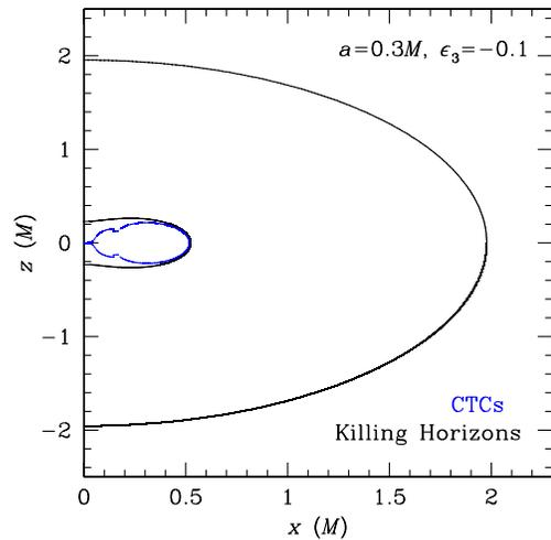
FIG. 12 (color online). Inner and outer Killing horizons and regions with closed timelike curves in the MK metric for  $a = 0.3M$  and  $\epsilon_3 = -0.1$ . The metric is regular outside of the outer Killing horizon, which is singular and located just outside of the null surface. Regions with closed timelike curves occur only inside the inner Killing horizon.
