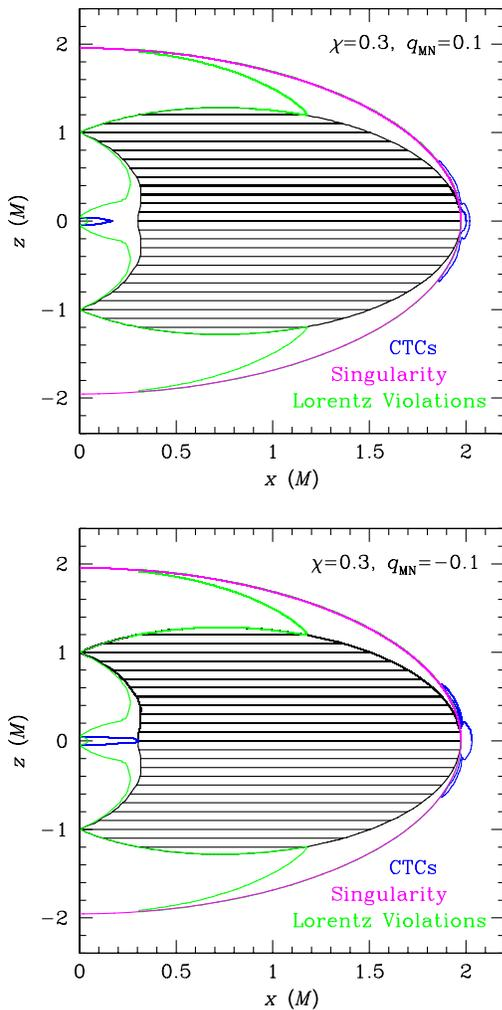
FIG. 10 (color online). Singularity and regions with Lorentz violations and closed timelike curves in the MN metric for  $\chi = 0.3$  and  $q_{MN} = \pm 0.1$ . Lorentz violations lie inside and closed timelike curves occur both inside and outside of the (singular) boundary that coincides to the event horizon of a Kerr black hole with the same value of the spin. In the black shaded region, the MN metric is imaginary.
