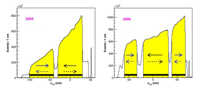
FIG. 2 (color online). Distribution of reconstructed vertex positions  $z_{vtx}$  along the beam axis for the target with two (left) and three (right) cells. Dark horizontal bars at the bottom mark the target fiducial regions, arrows denote the target polarization directions. See text for details.
