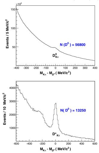
FIG. 4 (color online). Invariant mass spectra for the  $D_{K\pi}^0$  and  $D_{K\pi}^*$  samples with the approximate number of  $D^0$  mesons above background. Events in the spectra fulfill all the cuts in Table IV. The structure visible at about  $-250 \text{ MeV}/c^2$  is due to events with  $D^0 \rightarrow K^- \pi^+ \pi^0$  decays with the neutral pion not reconstructed in the analysis.
