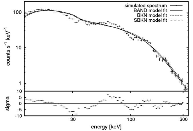
FIG. 2. Simulated femtolensed spectrum fitted with the BAND model. The fit has  $\chi^2 = 752$  for 75 d.o.f. The fit parameters are:  $A = 0.36 \pm 0.01 \text{ ph s}^{-1} \text{ cm}^{-2} \text{ keV}^{-1}$ ,  $E_{\text{peak}} = 174 \pm 5 \text{ keV}$ ,  $\alpha = -0.8 \pm 0.02$ , and  $\beta = -2.4 \pm 0.1$ . The smoothly broken power law (SBKN) model fit is almost indistinguishable from the broken power law (BKN) model fit.
