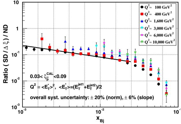
FIG. 18 (color online). The ratio of diffractive to nondiffractive dijet event rates as a function of  $x_{Bj}$  (momentum fraction of parton in the antiproton) for different values of  $Q^2 \approx \langle E_T^* \rangle^2$ . The quoted overall systematic uncertainty of  $\pm 20\%$  is due to the uncertainties  $\Delta \mathcal{R}_0$  and  $\Delta r$  listed in Table III.
