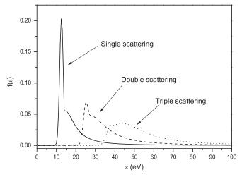
FIG. 3. The shape of the electron energy loss spectrum in tritium [10]. Different curves correspond to electron single, double, and triple scattering.
