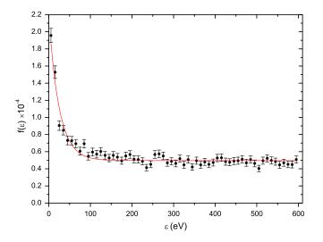
FIG. 5 (color online). Energy loss spectrum,  $\varepsilon = E_{in} - E_{fin}$ , for electrons which were trapped in the WGTS but after scattering reached the spectrometer. The bin size is 10 eV. The solid line is the analytic approximation of the losses.
