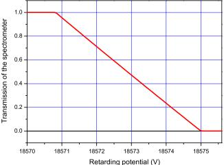
FIG. 6 (color online). Resolution function for electrons with energy of 18 575 eV. The curve corresponds to the magnetic field ratio  $B_A/B_0 = 2.26 \, 10^{-4}$ .
