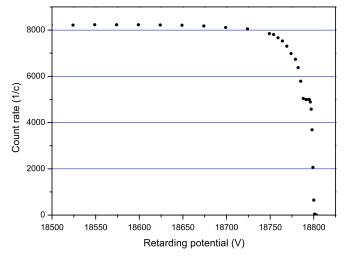
FIG. 4 (color online). Integrated spectrum from the electron gun versus the applied potential on the spectrometer electrode. The WGTS pipe is filled with tritium. The voltage on the electron gun cathode is around 18 800 V.
