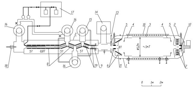
FIG. 1. Diagram of the installation: 1, 2—vacuum volume; 3, 4—electrostatic system; 5—ground electrode; 6–9—superconducting coils; 10—warm solenoid; 11—Nitrogen shield; 12—Si(Li) detector; 13—emergency valve; 14—magneto-discharge pump; 15, 16—mercury diffusion pumps; 17—tritium purification system; 18—electron gun; 19—argon trap.
