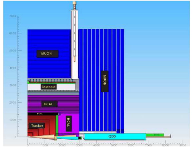
FIG. 1 (color online). Disposition of subdetectors in the SiD quadrant. All dimensions are in mm.
