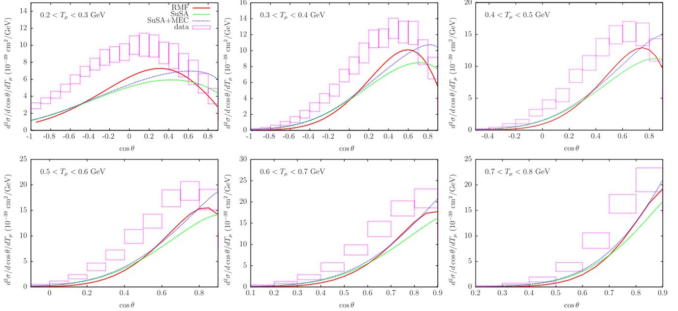
FIG. 4 (color online). Double-differential  $\nu_\mu$  CCQE cross section for  $^{12}\text{C}$  integrated over neutrino flux versus the outgoing muon scattering angle for various bins of the muon kinetic energy  $T_\mu$ . Results are given for RMF (red lines), SuSA (green), and SuSA + MEC (blue).
