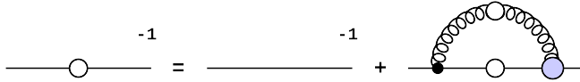
FIG. 9 (color online). The Dyson-Schwinger equation for the quark-propagator is shown. Specification of the fully dressed gluon propagator (wiggly line) and quark-gluon vertex (shaded blob) defines the truncation scheme.
