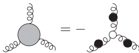
FIG. 1. Expression of the gluon three-point function [Eq. (38)] by means of three-point proper vertex function and propagators. Here and in the following, fat shaded gray blobs represent full Green's functions, small filled dots connected Green's functions, and small empty dots proper vertex functions.
