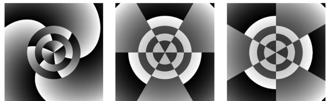
FIG. 1. Transverse phase distributions of the helical (left panel), vertically symmetric sinusoidal (center panel), and vertically antisymmetric sinusoidal (right panel) \text{LG}_{33} modes. The color represents the phase, in a range from 0 (white) to 2\pi (black).
