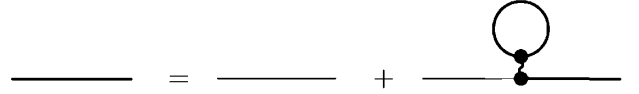
FIG. 1. Dyson-equation for the Hartree quark propagator (bold lines). Thin lines represent the bare propagator, the wavy line the bare interaction.
