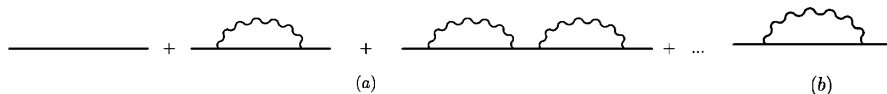
FIG. 1. Fermion propagator in the chain approximation, within the two-body Fock space truncation (a) and an irreducible contribution to the perturbative self-energy (b). Solid and wavy lines correspond to fermions and bosons, respectively.
