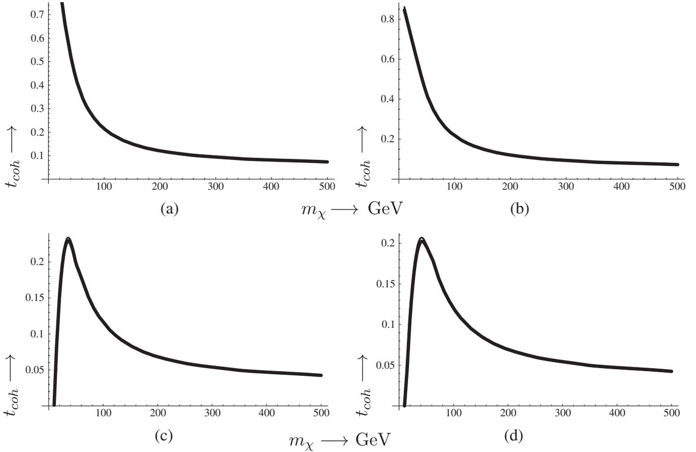
FIG. 9. The same as in Fig. 6 in the case of the target  $^{127}\text{I}$ . Now at the bottom the results shown correspond to  $Q_{\text{thr}} = 10$  keV. The dependence on the asymmetry parameter  $\beta$  is not visible.
