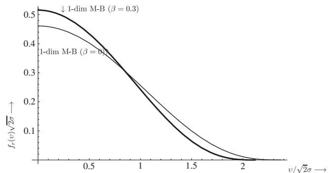
FIG. 1. The normalized velocity distribution in the radial direction  $f_r(v)$  ( $v = v_r$ ) for  $\beta = 0$  as a function of  $v/\sigma_r\sqrt{2}$  for  $q = 3/4$  (thin line) and the one-dimensional M-B distribution (thick line). For  $\beta = 0$ ,  $\sigma = \sigma_r$ . Since this one-dimensional distribution is symmetric, only the sector  $v \geq 0$  is shown.
