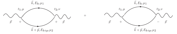
FIG. 1. The two diagrams contributing to the retarded self-energy for the photon at one loop.
