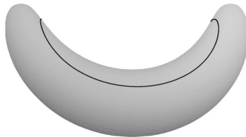
FIG. 1. This picture shows the “croissant” surface. A solid line separates two regions with opposite signs of the Gauss curvature. Each of these regions has the topology of a 2D ball. The Gauss curvature is negative in the upper ball-region.
