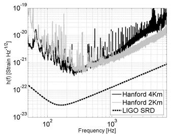
FIG. 2. Typical LIGO Hanford sensitivity curves during the S2 Run [strain  $Hz^{-1/2}$ ] (black and gray lines). The LIGO design sensitivity goal (SRD) is also indicated (dashed line).
