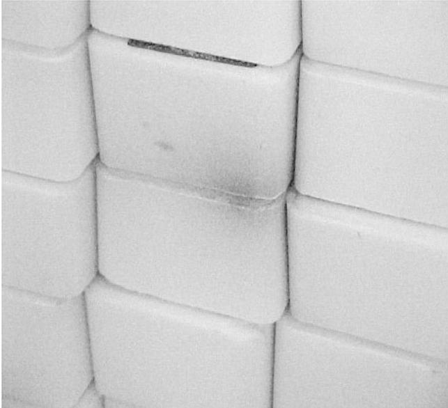
FIG. 8. The exit point of the beam in the downstream wall of the salt target, outlined by discoloration of the salt produced by beam and showing in cross section at the exit surface. Even at this location of order 15 radiation lengths along the shower, the shower core is still only several cm across (the salt blocks are 6 by 10 cm here in cross section).
