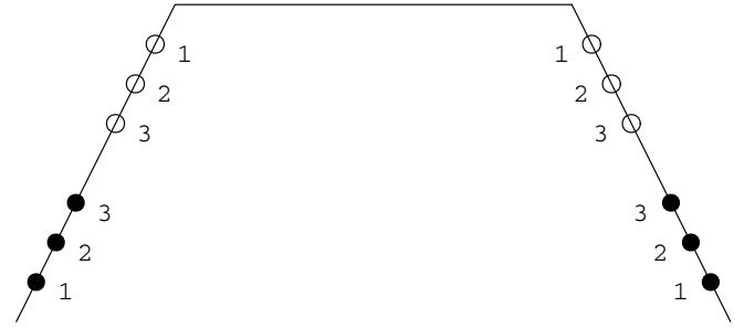
FIG. 10. A schematic graph of the starting points of bounce solutions to our linear toy model. Closed circles represent solutions which move outward as H is decreased, and open circles represent solutions which move inward. The numbers next to the points represent the number of times the solution crosses the top of the potential barrier.
