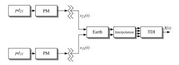
FIG. 5. Post-processed implementation of TDI combination X(t).
