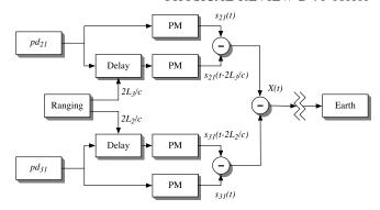
FIG. 4. Real-time TDI, in which the delays must be known at the time of measurement, and the TDI combinations are computed before transponding to Earth. TDI combination X(t) shown [Eq. (8)].
