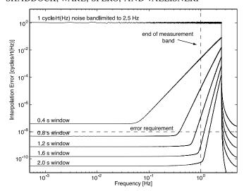
FIG. 3. Amplitude spectral density of interpolation error for Lagrange filters, shown with the spectral density of the initial 2.5 Hz-bandlimited noise. Spectral density is estimated by a triangle-windowed, averaged periodogram.
