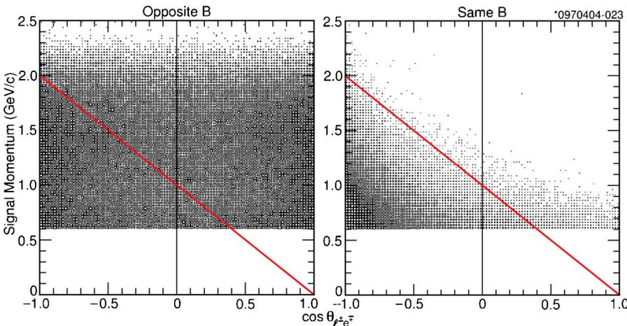
FIG. 1. Monte Carlo simulation of electron momentum versus the cosine of the opening angle between the tag lepton and the signal electron ( $\cos \theta_{\ell e}$ ) for unlike-sign dilepton pairs from opposite  $B$ 's (left) and from the same  $B$  (right). The line indicates  $p_e + \cos \theta_{\ell e} = 1$ .
